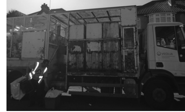
Traditional 12-tonne 'stillage' vehicle with variable-height, internal- and external-, double-sided loading (no capacity for bulk bins)
